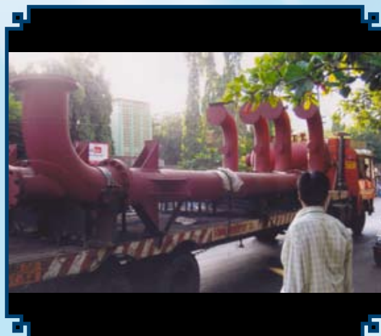
EDC Reactor with mixing nozzle Client : Chemplast Sanmar Ltd
