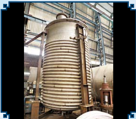
20 M3 Reactor with Limpet Coil Client : Bayer Crop Science Ltd
