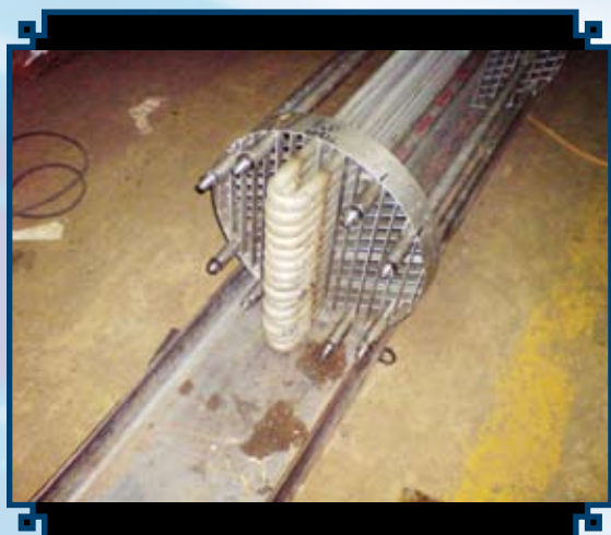
'U' Bundle Exchanger under assembly
