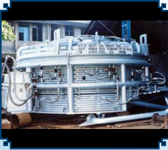
Water cooled Laddle roof Arrangement Client: Indomag Steel Technology
